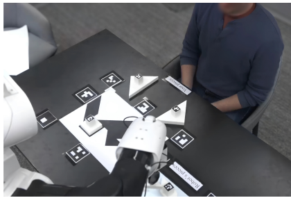
(a) Freezing failure: the robot pauses mid-action while holding a puzzle piece.
