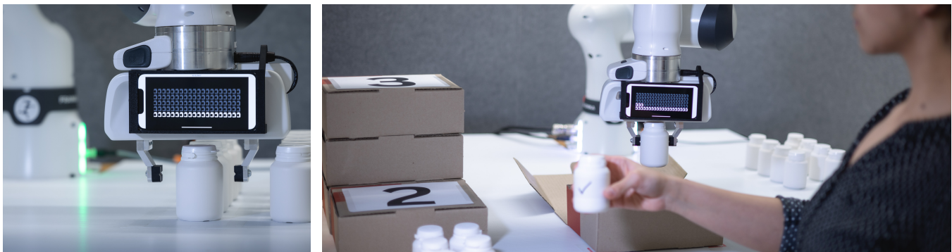
Figure 1: (left) The robot conveys low confidence in a pill box using a GUI before picking up the pill box. (right) The robot and the human pack their pill box into the package on the working station during a human-robot collaboration task.
