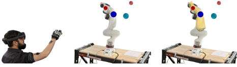
Fig. 5: Study 2: participant, condition NO ARM and AR ARM. Blue and red sphere rendered on elbow and wrist respectively. Lighter blue and red denote targets to match posture.
