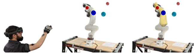
Figure 10: Study 2 (left to right): Participant; Condition of no visualisation of AR arm on robot; Condition with visualisation of AR arm on robot. Blue and red sphere rendered on elbow and wrist respectively. Lighter blue and red denote targets to match posture.
